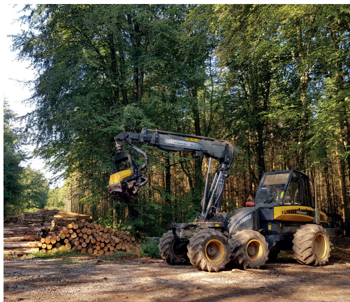
Figure 2. Conserve existing carbon stocks during harvesting operations by avoiding ground disturbance and soil compaction wherever possible. (Photo: © Crown copyright, Forest Research)
