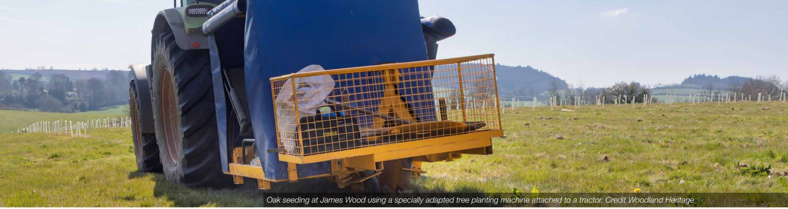
Oak seeding at James Wood using a specially adapted tree planting machine attached to a tractor. Credit Woodland Heritage
