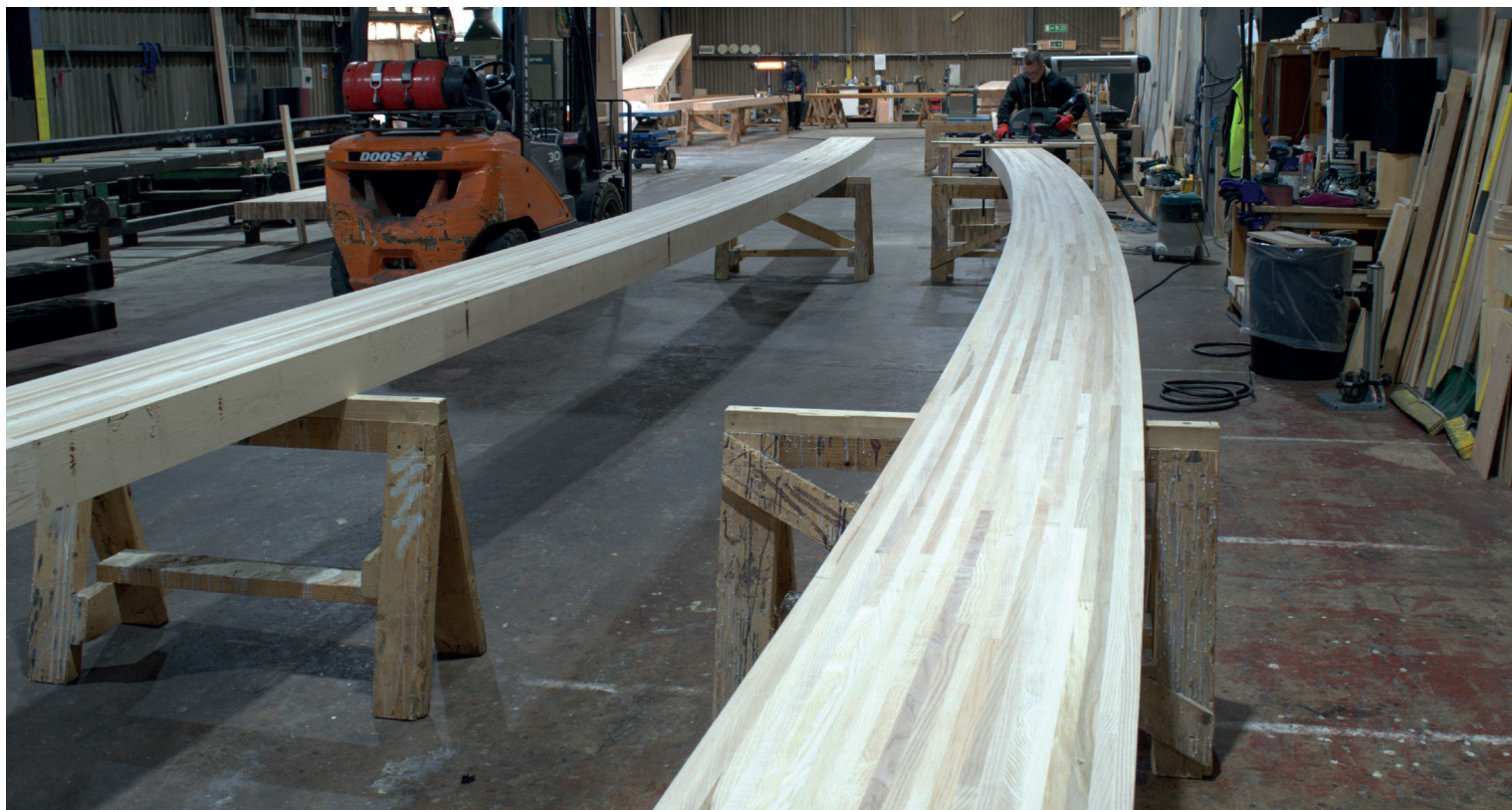
Figure 6. Home grown and manufactured ash glulam beams, Buckland Timber, CREDITON, Devon.
