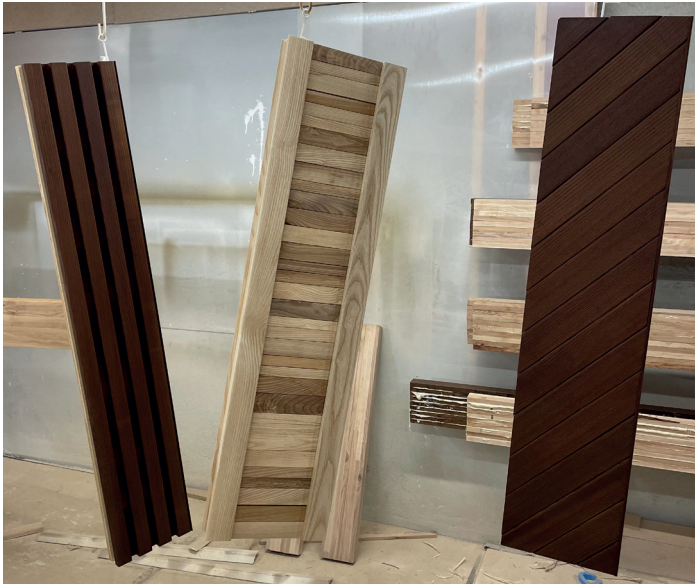
Figure 3. Different lamination patterns of TMT and ash at Scandinavian Timber.
