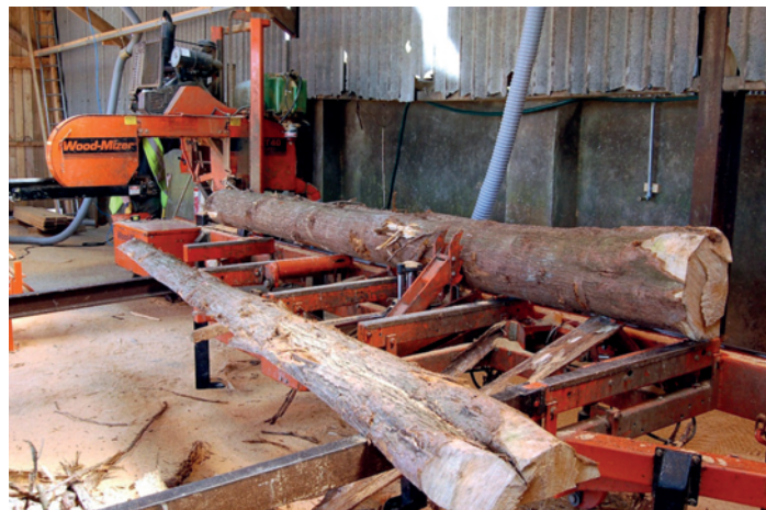
Figure 3b. Processing western red cedar for cladding boards, Cornwall. (Photo: Scott McG Wilson)
