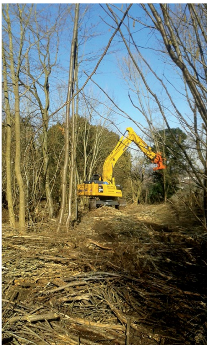
Tree shears are used for soft felling of ash trees
